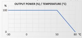
Thus if the charger is forced to operate in an environment above +50°C, it will simply reduce its output power to the corresponding value in the above chart and continue normal operation.
